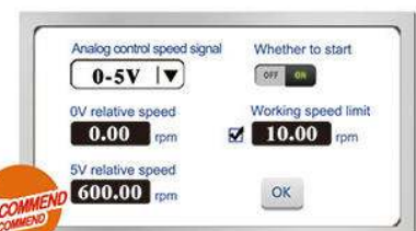
External Control Speed Setting Interface
