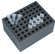
(2) "BLC570" 0.5ml Centrifuge Tube x 63 holes
