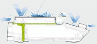
In case of a liquid overflow a built-in drainage protects the electronic components of the device.
